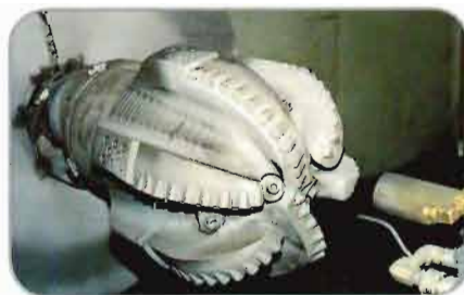
Drill bits receive a coating application from PAS Technologies' detonation gun, licensed by Praxair Surface Technologies.
